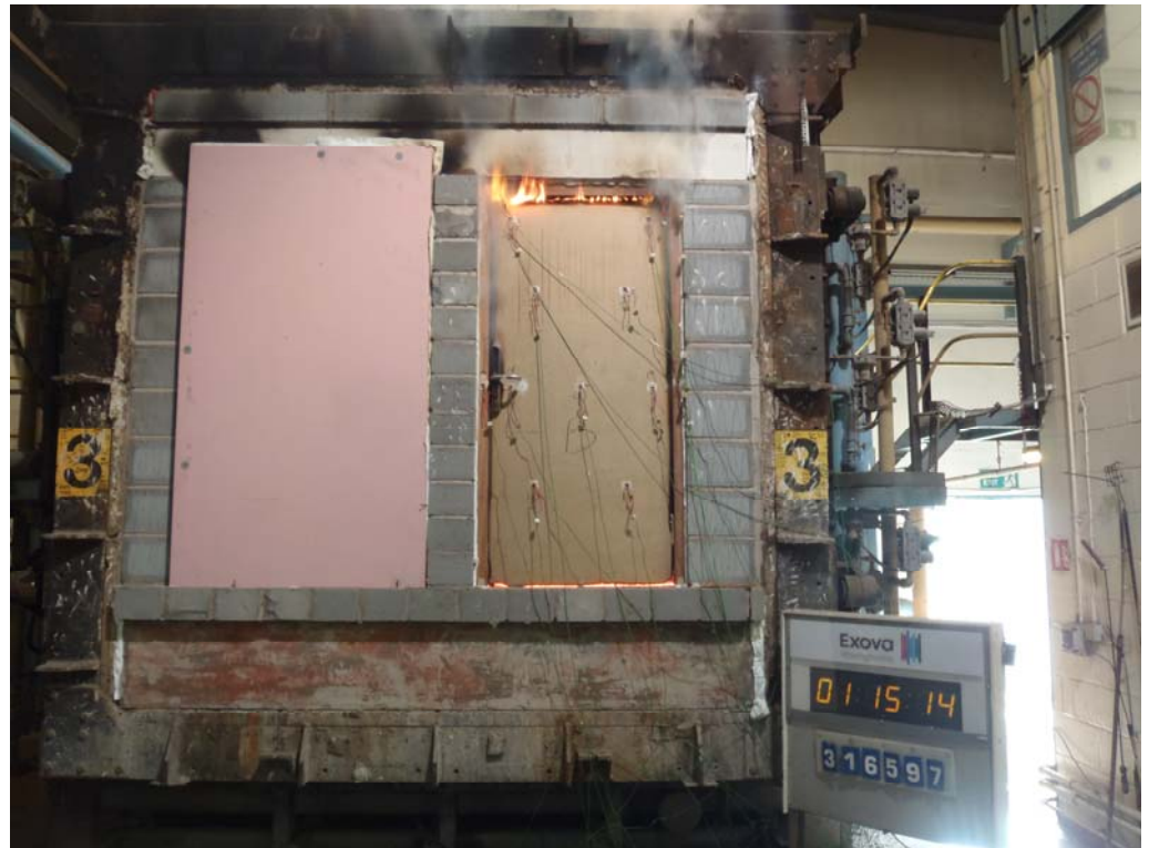
Flaming seen across the head of Doorset B after a test duration of 75 minutes
