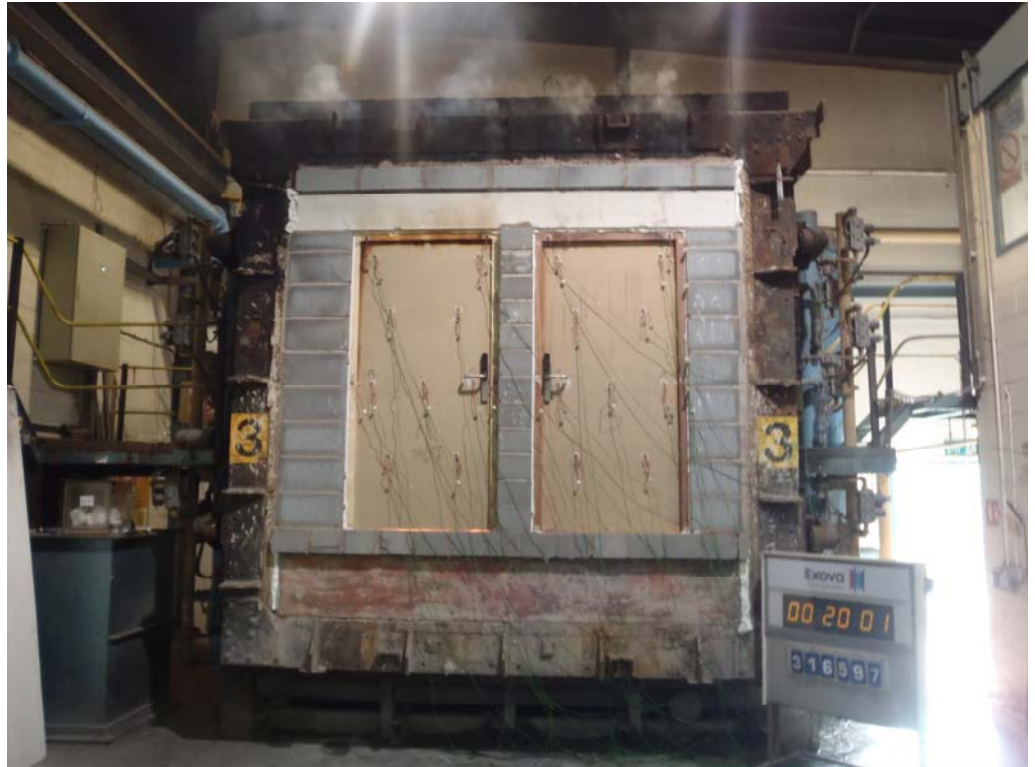
The unexposed face of the doorsets after a test duration of 20 minutes
