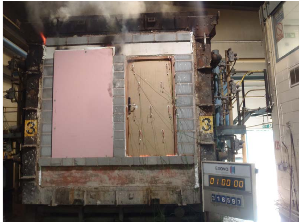
The unexposed face of the Doorset B after a test duration of 60 minutes
