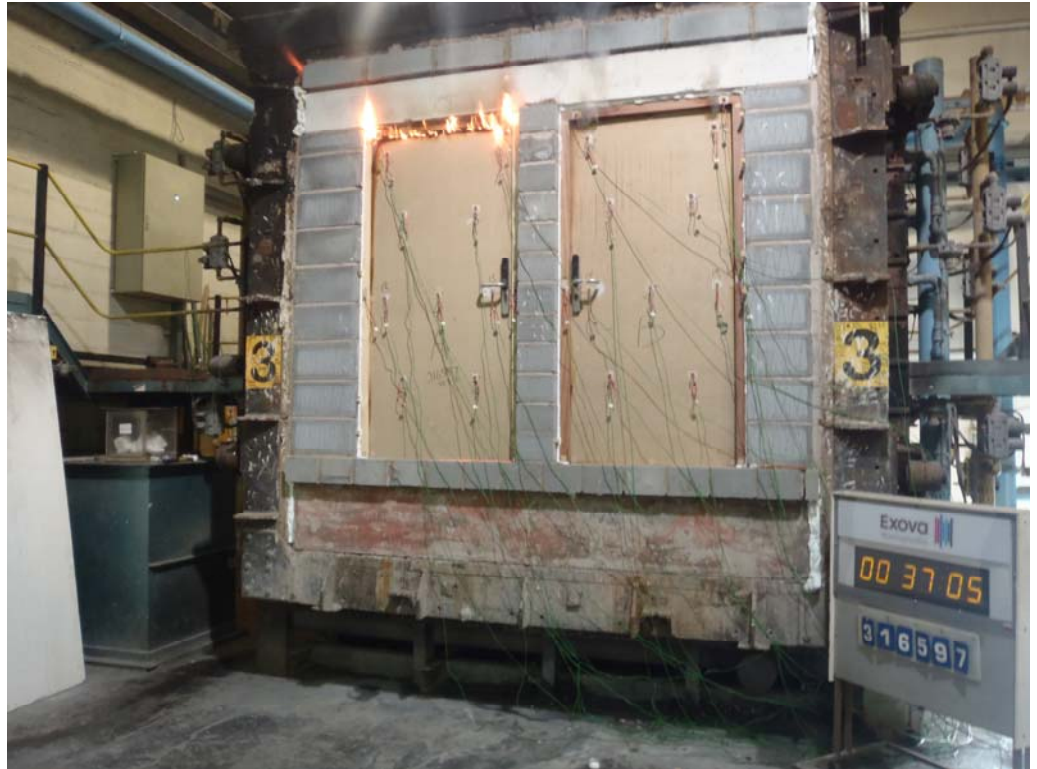
Flaming seen across the head of Doorset A after a test duration of 37 minutes
