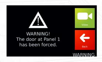
Alarm messages will display to the user at the monitor if the option has been set in the local Installer screen.
