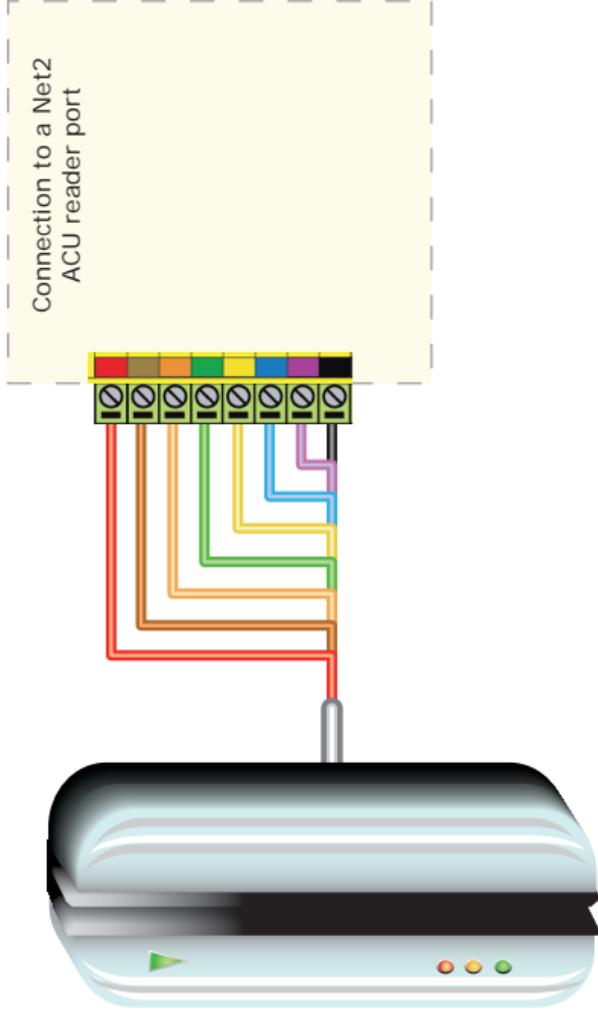
WHITE labelled control units provide 5V at the Red terminal. The Red power wire for the reader should therefore be directly connected to the 12V supply terminal.
