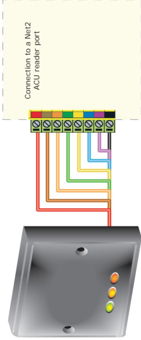
WHITE labelled control units provide 5V at the Red terminal. The Red power wire for the reader should therefore be directly connected to the 12V supply terminal.
