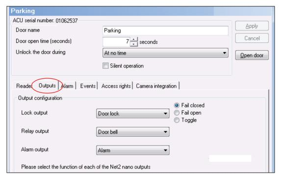
Lock output - This is a transistor 'open drain' output, (not a voltage free contact) that has been designed to simplify the wiring of the lock. It can be configured to operate in Fail lock, Fail unlock or toggle modes and removes the need for additional links or diodes normally required when using a relay for output switching. Relay output - This provides a set of volt free contacts to switch external devices.
