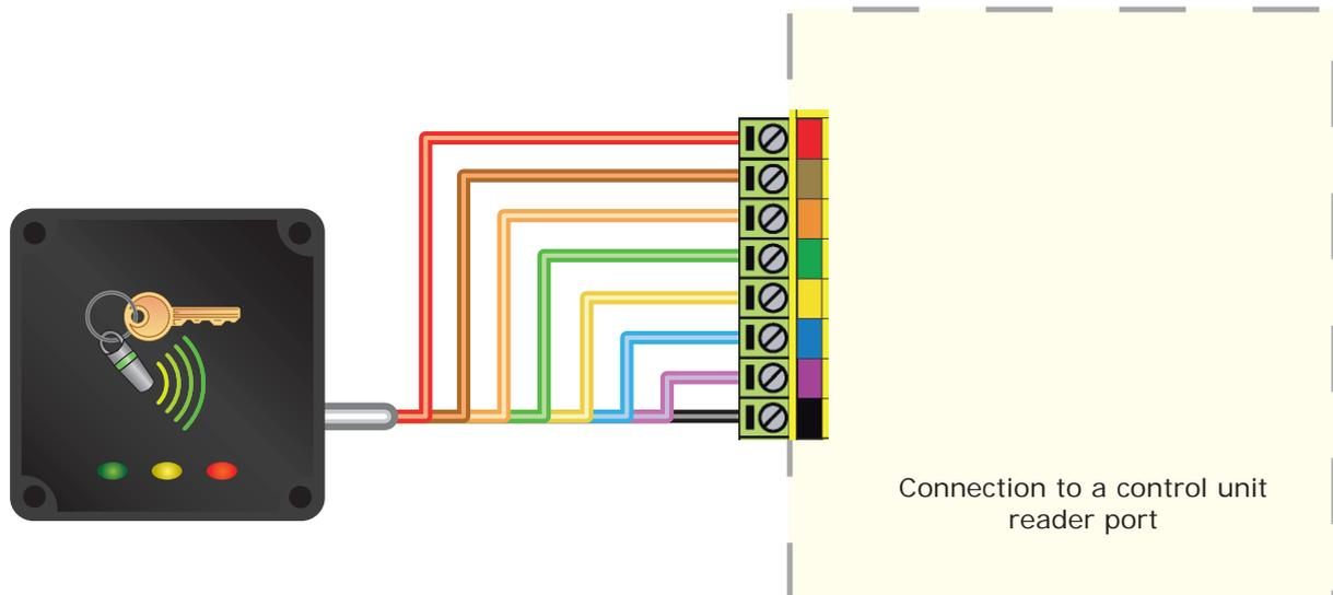
WHITE labelled control units provide 5V at the Red terminal. The Red power wire for the reader should therefore be directly connected to the 12V supply terminal.
